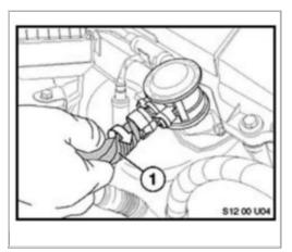
Visually inspect the non-return valve fitting internally for carbon type contamination. (Twisting the corner of a clean shop rag into the valve fitting as shown will assist with this check.)
