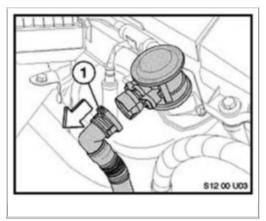
Disconnect the air pump feed line/hose (1) at the non-return valve (line from the secondary air pump
